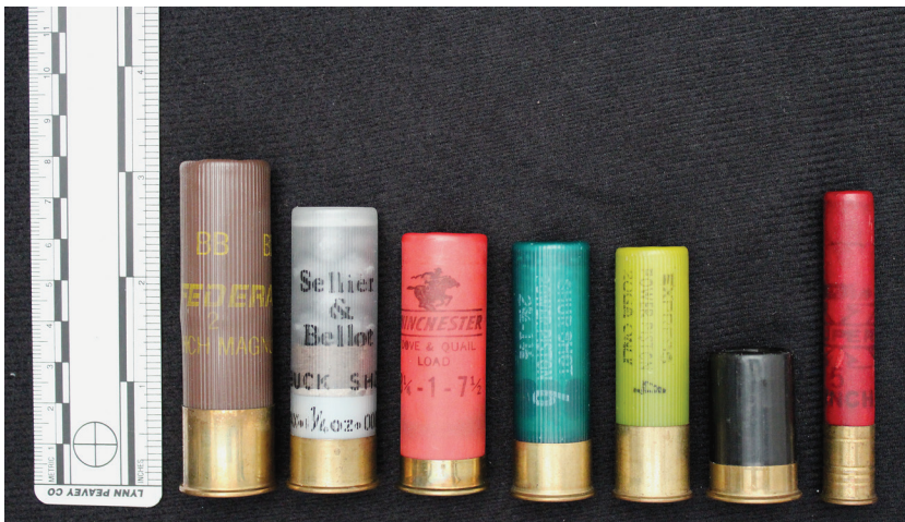
Figure 2.3 A cross-section of various size shot shells, from left to right: 12-gauge 3½" Super Magnum, 12-gauge 3" Magnum, 12-gauge 2¾", 16-gauge 2¾", 20-gauge 2¾", Aguila 12-gauge 1½", and .410 3" shell. (Images from author's collection.)
